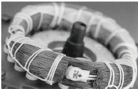
Fig. 21 Motor with Thermal Switches (PTO)
